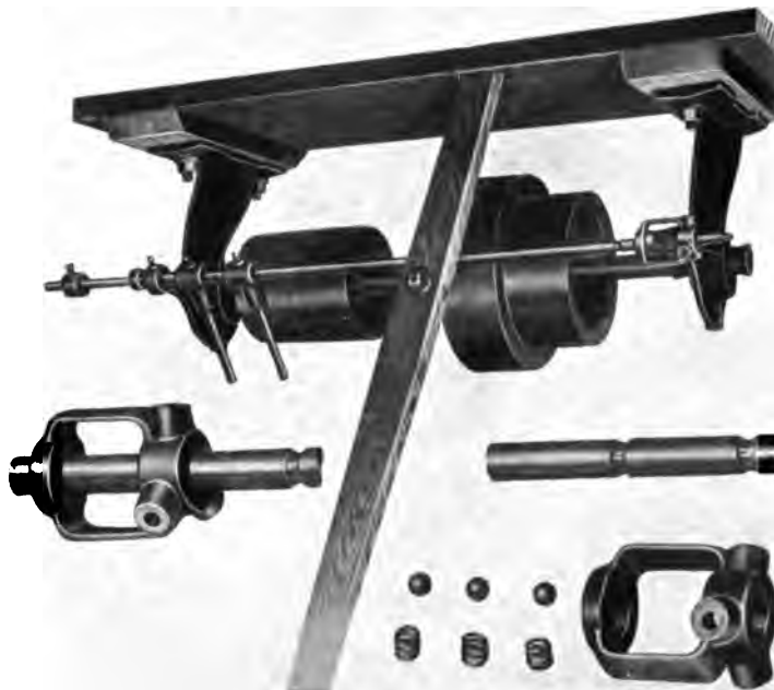
Fig. 1. Locking Shifter for Counter-Shaft. (Pat.)
